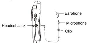
**Note:** When the headset is plugged into the headset jack the microphone on the handset will be deactivated.
